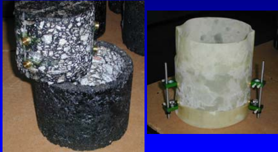
150 mm tall by 100 mm diameter, cored from SGC
